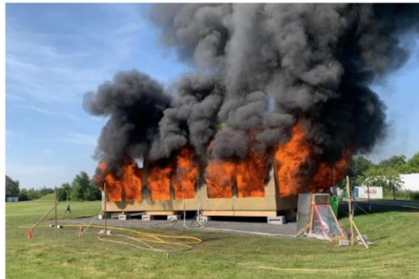
Mass timber structure during the fully developed fire.
